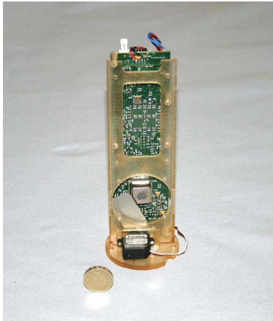
Figure 6: Photograph of prototype sensor unit.
