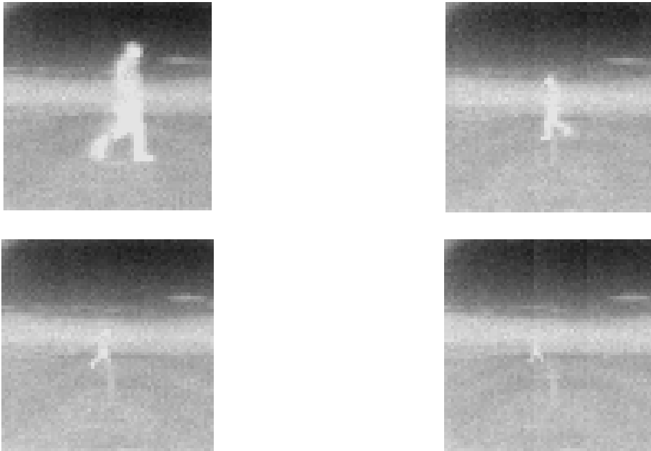
Figure 8: Example imagery of a walking man using 10° field of view (1" focal length) lens.
